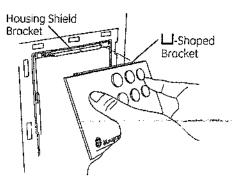
Angle to top of board into the tabs on housing shield bracket. Snap board into place.
