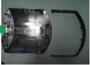
Replace either part and fix them by the same screws. (Tightening Torque:  $0.8 + /-1 0.1 \text{ N} \cdot \text{m}$ ) Since they are tapping screws, tighten them along the existing threads.
