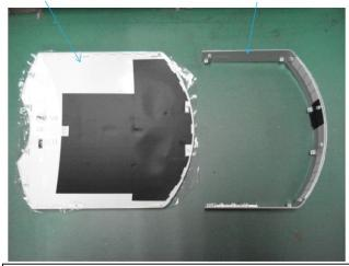
Replace either part and fix them by the same screws. (Tightening Torque: 0.8 +/-1 0.1 N • m) Since they are tapping screws, tighten them along the existing threads.
